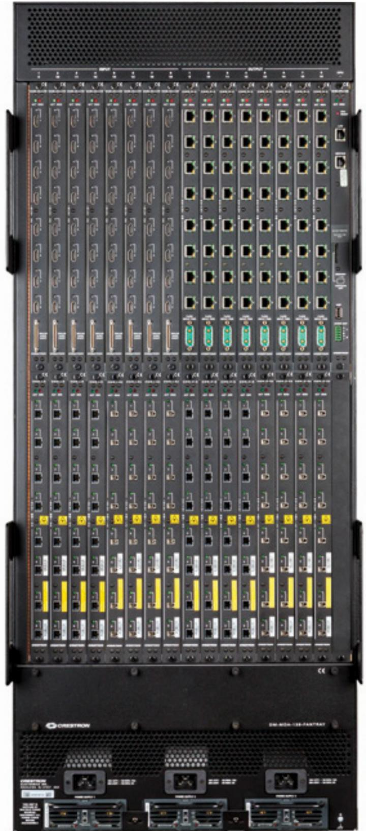
DM-MD128X128 – Rear view with I/O blades installed
